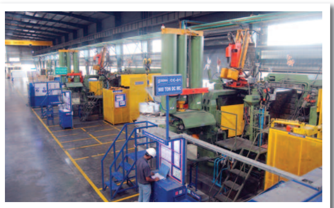
Environment friendly Die casting - Honeywell AC250 Cold Chamber (Zitai - 900 Ton)
